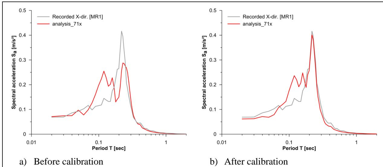
Figure 6. Comparison of response spectra before (a) and after (b) calibration in x-direction at sensor no. 1 (channel 1)
