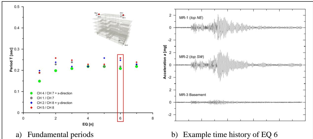
Figure 4. Instrumentally derived fundamental periods of the study building (a) and recorded response caused by one of the strongest earthquake during the operation time (b)
