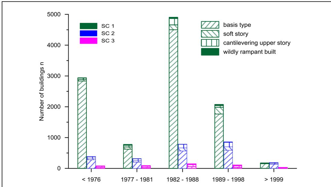
Figure 3. Distribution of the reinforced concrete structures according to the story class, building type and construction period.
