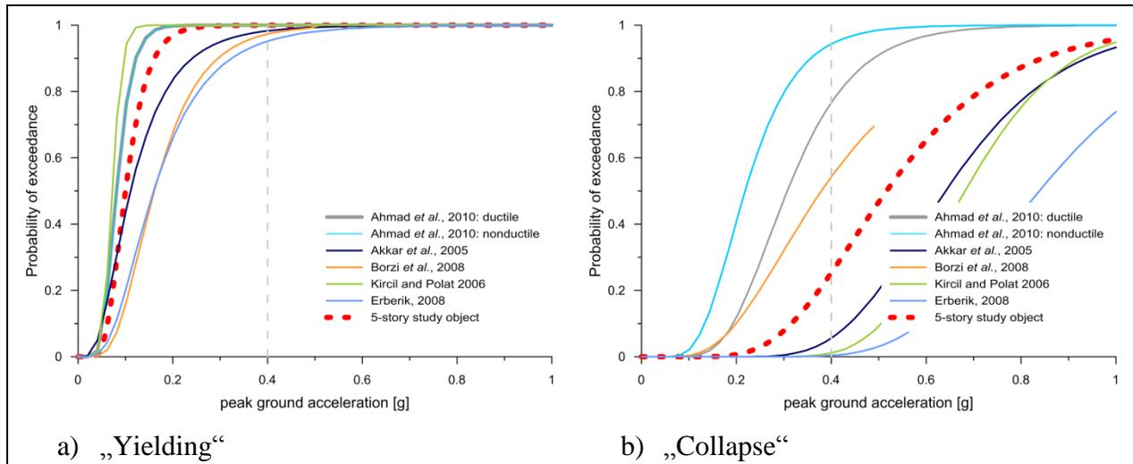
Figure 7. Comparison of fragility functions proposed for 5-story R.C. frame structures with masonry infill walls for different limit (performance) states; definitions acc. to [9].
