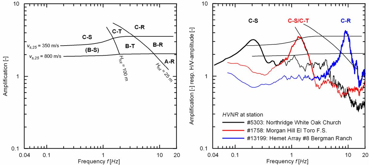
Figure 1. (a) Qualitative ranges of possible peak locations of one-dimensional transfer functions for site classes of DIN 4149: 2005 (b) overlain with spectral H/V-ratios on microtremors recorded at selected Californian strong motion sites showing soft soil conditions but different sediment thicknesses.
