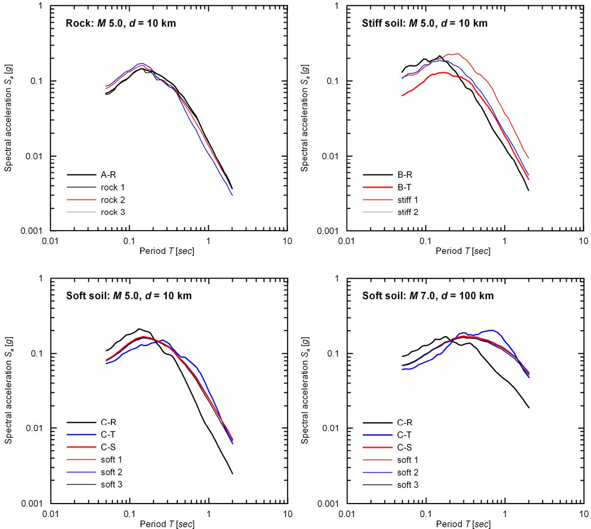
Figure 7. Comparison of predicted spectral acceleration for Type I\* with Type II datasets in order to illustrate the influence of record number the regression rests upon. (Note: Spectra for soft 1, soft 2 and soft 3 are fully hidden by the respective C-S spectra.)
