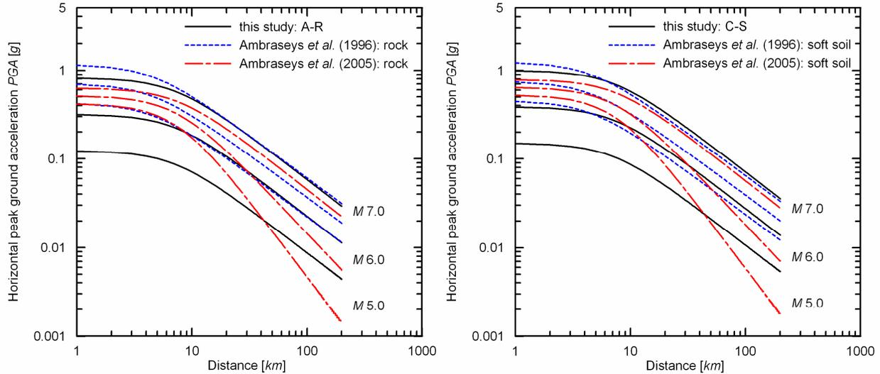
Figure 5. Comparison of attenuation curves for horizontal peak ground acceleration by Ambraseys *et al.* (1996), Ambraseys *et al.* (2005) with this study (Type II, entire dataset).
