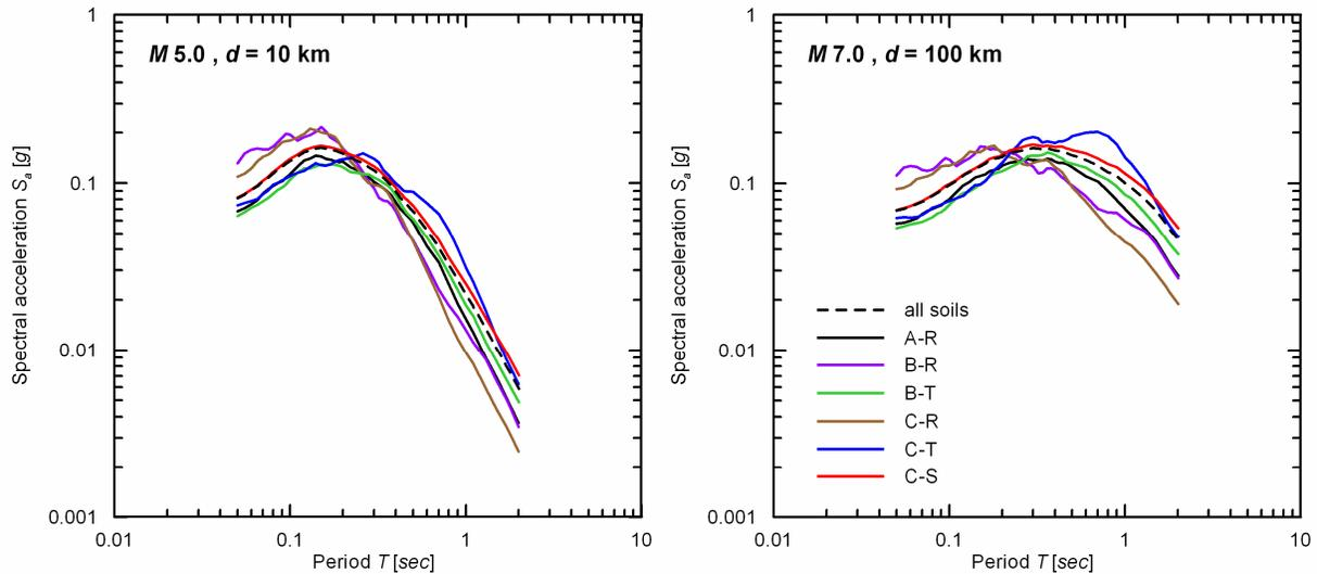
Figure 6. Comparison of predicted spectral acceleration for Type I dataset (“all soils”) with Type II datasets (site classes of DIN 4149: 2005).
