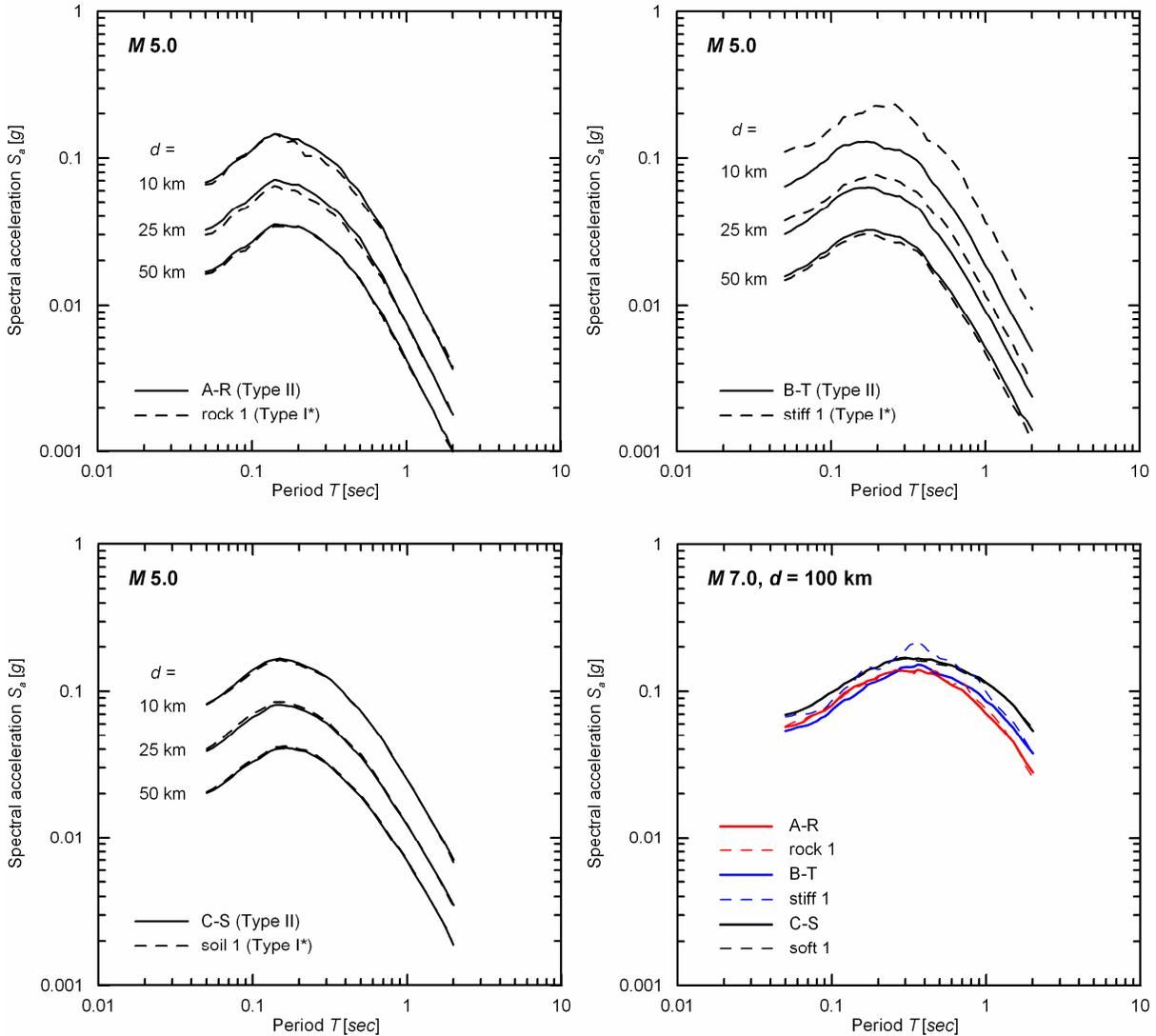
Figure 8. Comparison of predicted spectral acceleration for Type I\* with Type II datasets in dependence on distance  $d$ .
